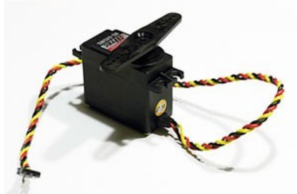
Higher quality, "extra strong" servo with twisted wires.
